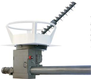
This 80° conveyor system suits silos from 3 to 8 m in diameter and all kinds of dry wood splints and chips up to size G 30 according to OeNORM W 1733. Especially for silo installations which are out of use for longer periods (i.e. only during heating seasons).
