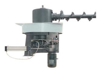
For silos up to 8 m in diameter and all kinds of dry wood splints and chips up to size G 30 according to OeNORM M7133. The auger is driven by compressed air, so no additional hydraulic power unit is needed. Especially for silo installations which have to be emptied down to the floor.
